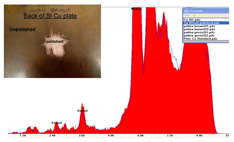
The red spectrum is the unpolished back side of the SI Cu plate. The blue spectrum is the polished spot on the back side of the SI Cu plate. One can see that the unpolished surface shows a trace of CI. The next slide shows the CI on an expanded scale.
