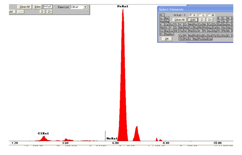
This is the difference between the brown patina and the polished back of the SI Cu sheet. Clearly the patina is composed of Fe and Cl
