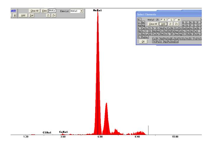
This is the difference spectrum of pure Cu and the SI Cu alloy. Clearly Mn and a trace of Fe are present in the SI Cu alloy.
