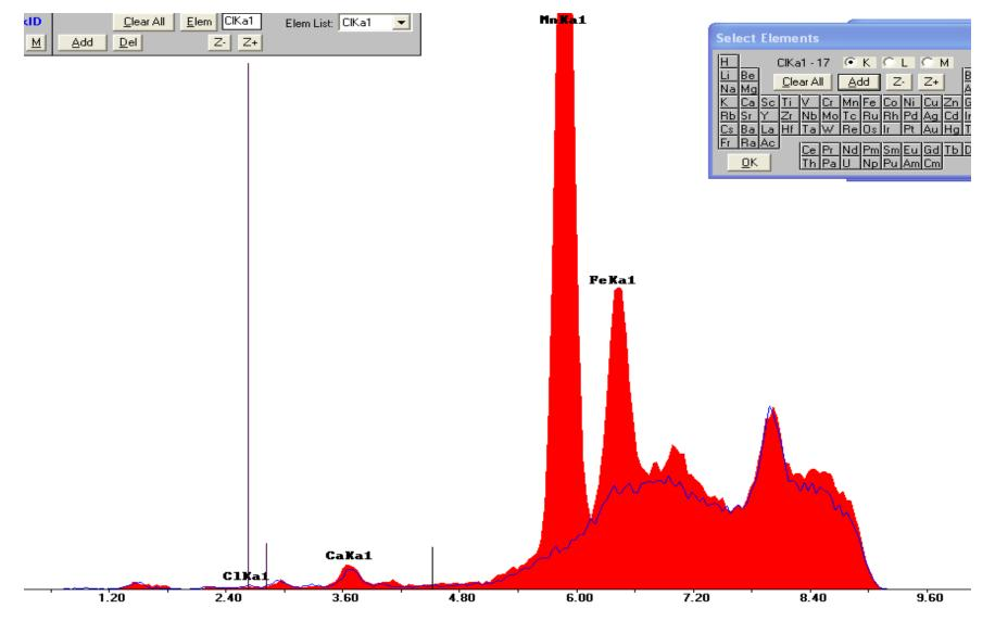
The blue spectrum is of pure copper the red spectrum is the Smithsonian Institute (SI) base material (polished with no patina). Using the instrument in alloy mode, it showed the base copper to be C65500-82A (1.02Mn/95.76Cu). A difference spectrum for these 2 spectra is shown in the next side.
