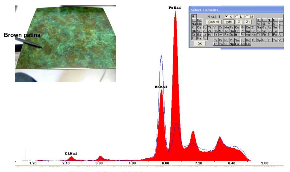
patina brownSI1 (red) /Cu SI1 (blue): Cu SI1 is the polished spot on the back of the plate, pure alloy. It is clear that the patina contains a large amount of Fe and some Cl. The red spectrum is the brown patina spot shown in the above picture.
