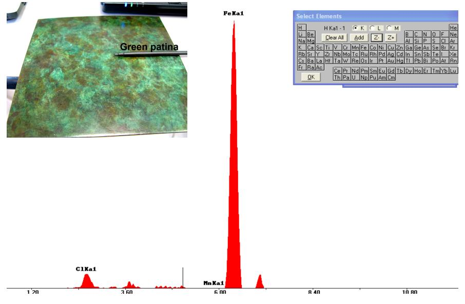
This is the difference between the green patina and the polished back of the SI Cu sheet. Clearly the patina is composed of Fe and Cl
