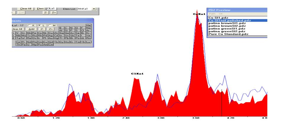
The red spectrum is the <u>unpolished</u> back side of the SI Cu plate. The blue spectrum is the <u>polished</u> spot on the back side of the SI Cu plate. One can see that the unpolished surface shows a trace of CI.
